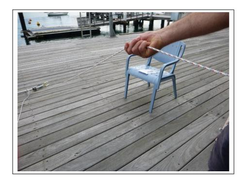
6. Go back to the gooseneck end of the boom. Grab both ropes as close as possible to the end. Make loops to end of both ropes.
